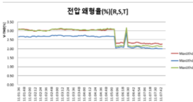
Figure 9 THDv at panel 2AHF-2A reduced by 16%
