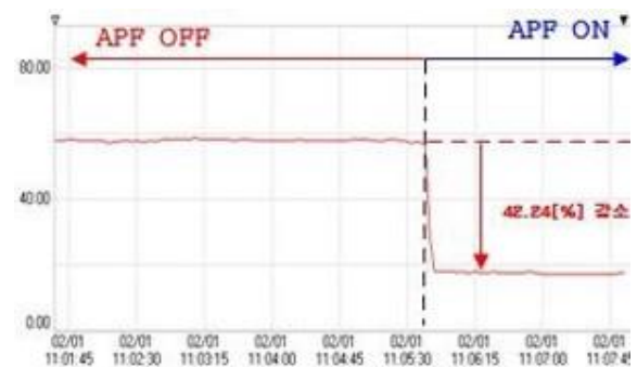
Figure 8 THDi at panel 2AHF-2A reduced from 59.60% to 17.36%
