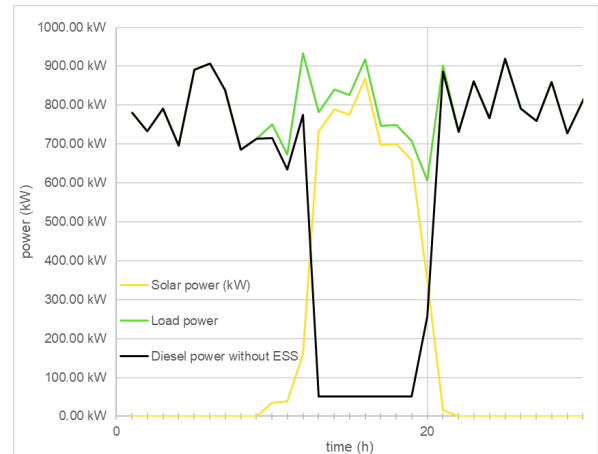
Figure 4 Solar generation capacity is limited by load level. DGS are used for power balance control.
